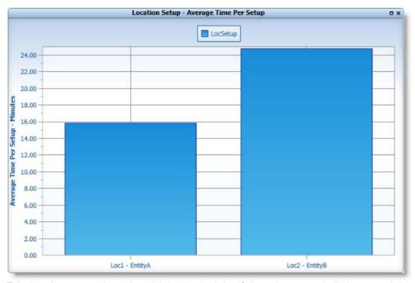
This chart shows setups data collected during the simulation. Column charts can only display one statistic at a time, this example shows Average Time Per Setup. Use the Statistics drop-down in the Filter Options panel to select other statistics to display.
