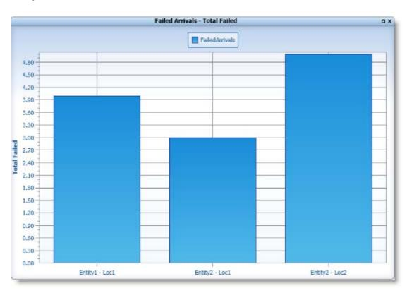
This chart shows the total number of failed arrivals, or the number of entities that failed to arrive at the specific location due to insufficient capacity.
