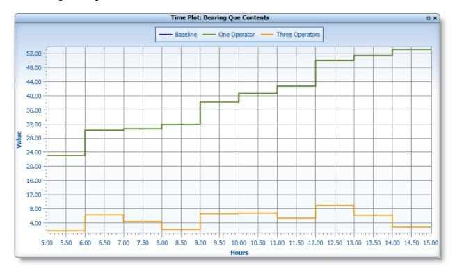
Time plots show performance values as they occur over time. This allows you to see trends and spikes in activity as the simulation progresses. Time plots can only be displayed, if the user has selected Time Series as the statistics type for elements in the model. The Time Plot: Bearing Que Contents example shown, shows the contents of the
