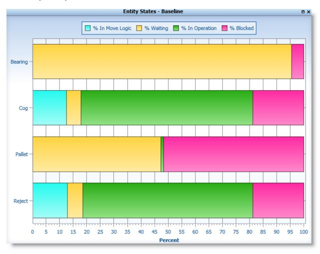
This chart shows a horizontal stacked bar chart summarizing the states of each entity type during the simulation run. States describe the condition of these objects.
