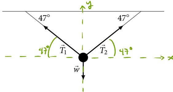
The tensions  $\vec{T}_1$  and  $\vec{T}_2$  both have a magnitude of 20lb. Find the magnitude of the weight  $\vec{w}$ .
